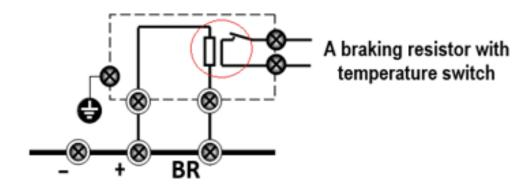
IS580T170~300 and IS580-2T170~300 require an optional external braking unit. More details of braking unit see following slides.
