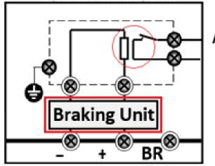
A braking resistor with temperature switch
