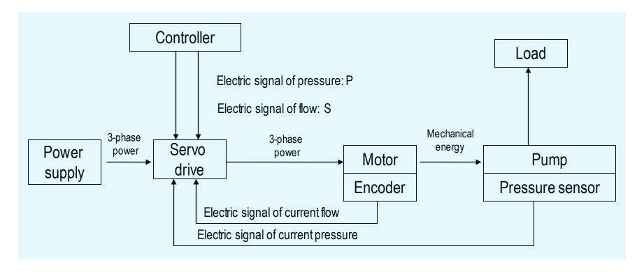
The Contact media between the controller and servo drive, and between the servo drive and other devices is electric signals. Different electric signals correspond to different pressure or flow values. For example, a pressure range of 0~250 bar corresponds to a voltage feedback of 0~10 V.
